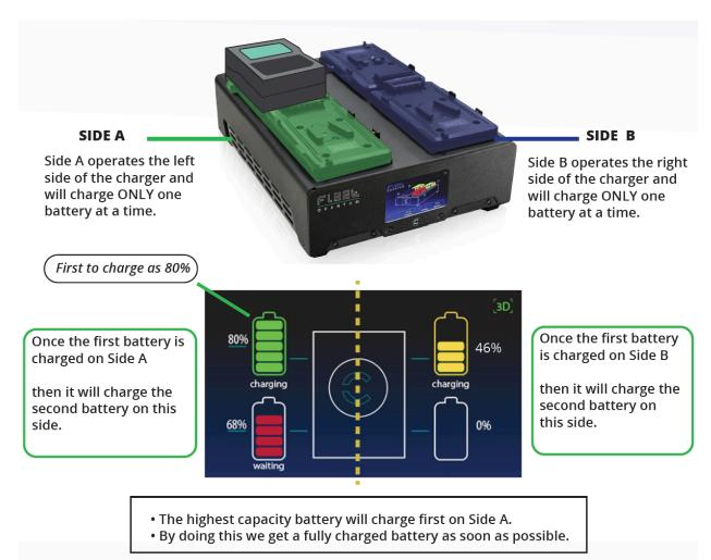
The charger has two independent charging circuits two address the left and right side of the charger(side A and B).
